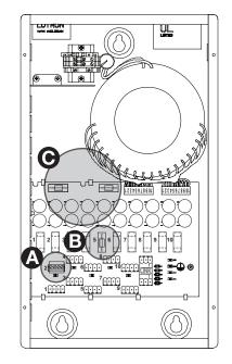
If an output status LED has turned off, the fuse will need to be replaced. The QSPS-P1-10-60 comes with two spare 5x20 mm 2.5A fuses.
